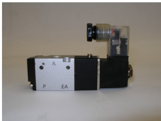
Figure 1: Model 3V110 with port labels shown.
